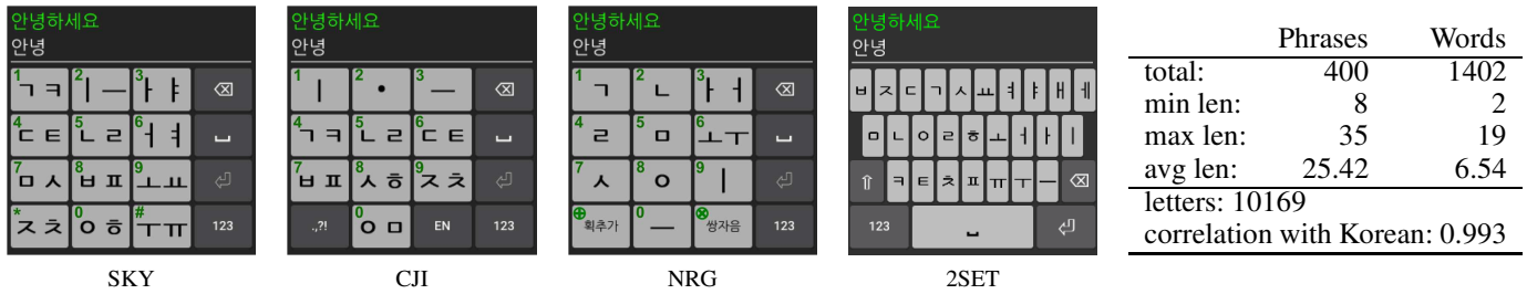
Figure 1. The four layouts used in this study and phrase set statistics; the numeric labels are only for reference and do not appear on the interface. The backspace key deletes only the last letter of the last syllable.
